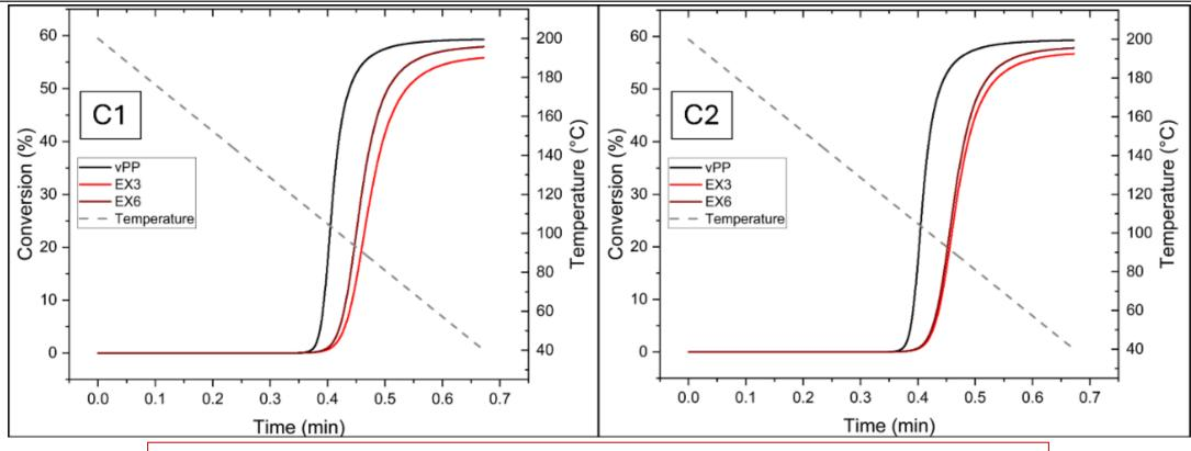
Simulated crystallization conversion profiles (200°C to 40°C in 40s)
