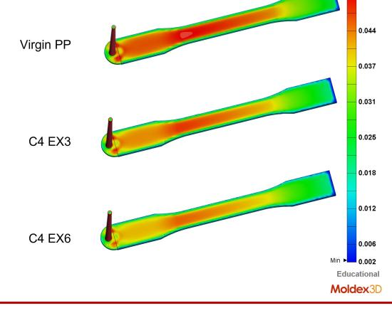
Injection molding simulation results for maximum shear stress
