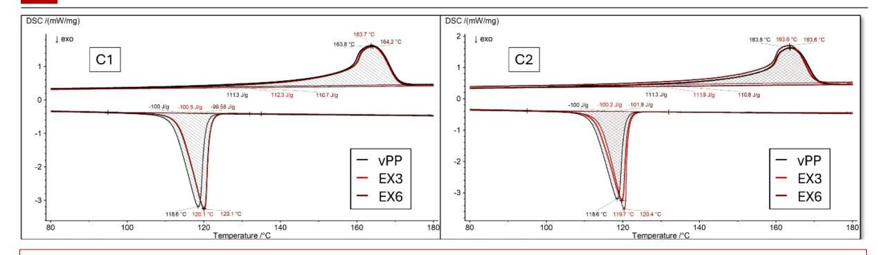
Non-isothermal DSC thermograms showing heating (top) and cooling (bottom) cycles at 10 K/min for virgin PP and EX3 and EX6.
