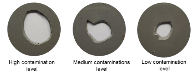
Multiaxial impact test acc. to ASTM D-3763 (2.2 m/s 23°C)
