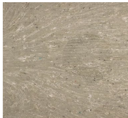
Silver streaks on part molded with green compound
