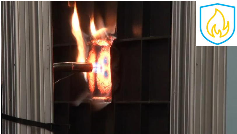
Final 20 seconds of 5.5-minute test @ 1100°C
