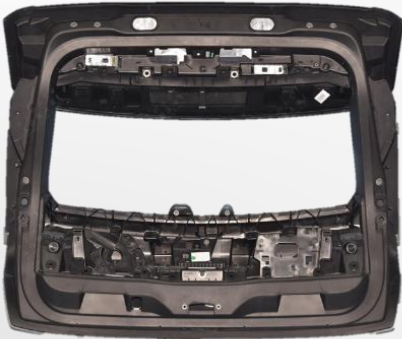
Structural and inner lifgate achieving in PP-GF40 ( THERMOFIL HP® F811X9X)
