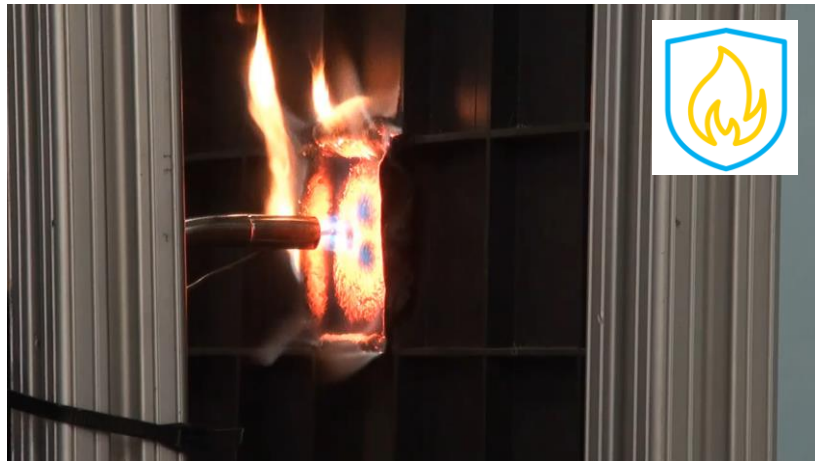
Final 20 seconds of 5.5-minute test @ 1100°C
