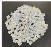
Although conventional polyamide resins, such as PA6 and PA66, exhibit excellent mechanical properties and heat resistance, their rapid crystallization often causes poor processability at injection molding.
