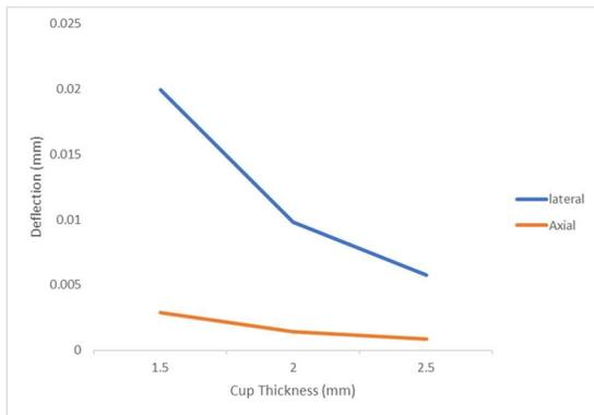
Figure 8: x and y - Deflection on 7.5mm Core thickness using P20 tool steel vs Cup thickness using a PP & PC of 5 g/min MFI pressure.
