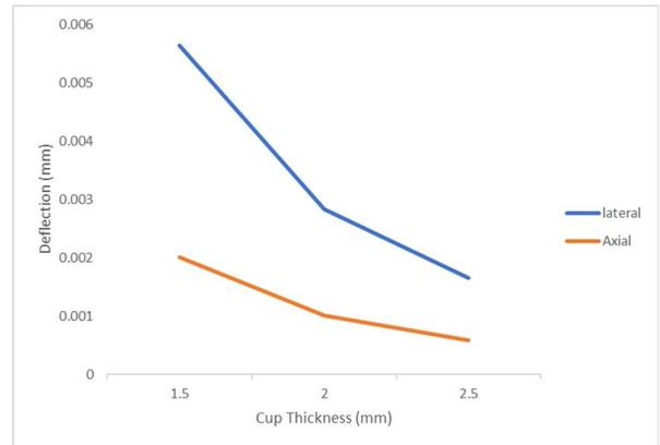
Figure 9: x and y - deflection on 10mm Core thickness using P20 tool steel vs Cup thickness using resin pressures for a PP & PC of 5 g/min MFI
