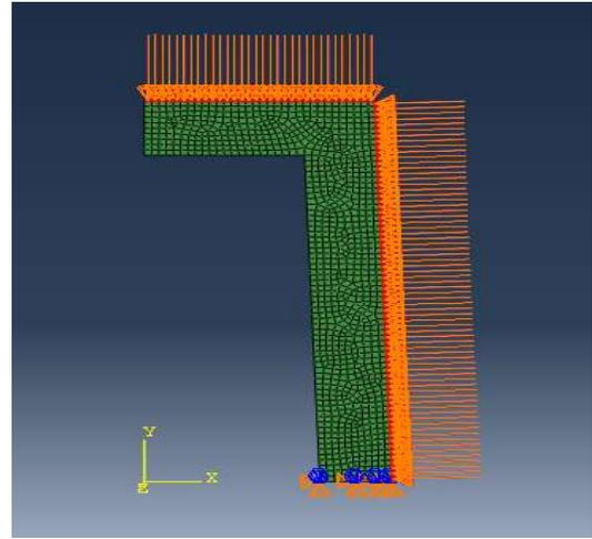
Figure 6: Core with applied boundary condition and pressure applied.
