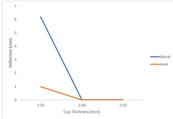
Figure 7: x and y - deflection on 5mm Core thickness using P20 tool steel vs Cup thickness using resin pressures for a PP & PC of 10 g/min MFI
