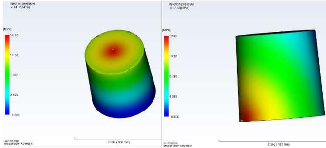
Figure 5: Injection pressure profiles with the gate location from the (a) top with wall thickness of 1.5mm using a PP plastic with MFI of 5 g/10min (b) bottom with wall thickness of 2mm using a PP plastic with MFI of 10g/10min
