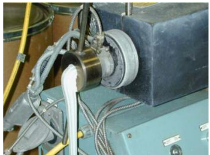
FIGURE 2 Purging TiO 2 masterbatch from debris fouled screenpack.
