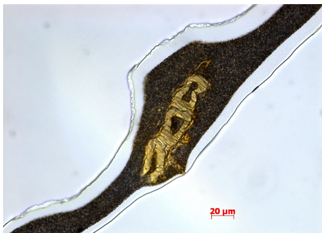
Figure 8. Transmitted bright-field image of PE film containing a fibrous gel.
