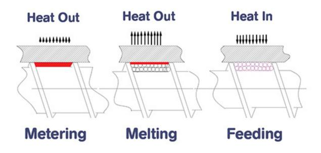
Generally, the first section of an extruder absorbs heat from the barrel; the middle or melting zones add heat to the barrel; and the last zones stay fairly neutral, adding some heat to the barrel.
