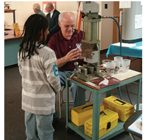
Visitors molding screwdrivers on a small manually operated molding machine. Material is PP.
