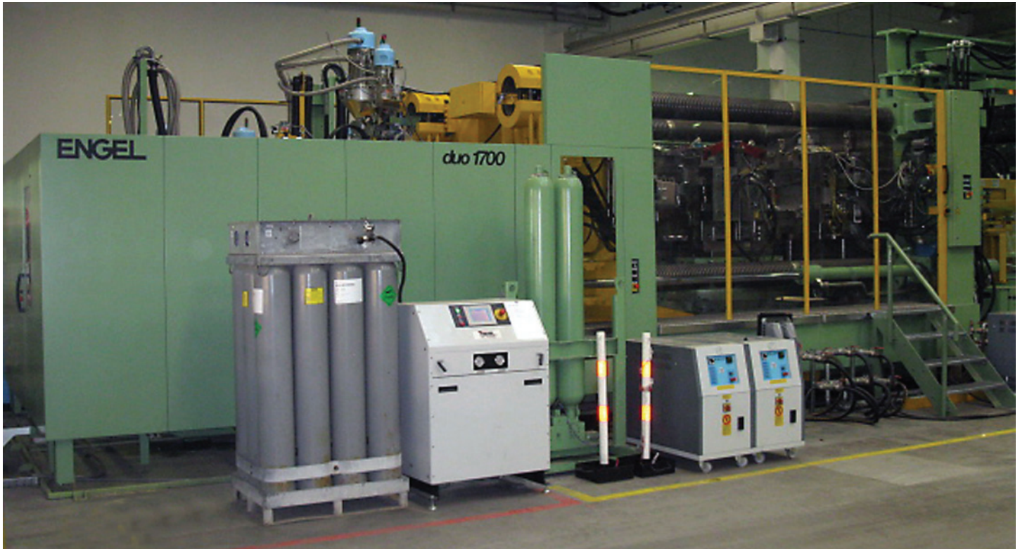
Figure 4: The production line manufactures cockpit covers with softtouch-surface in just a single process step. Figure courtesy of SOLE.
