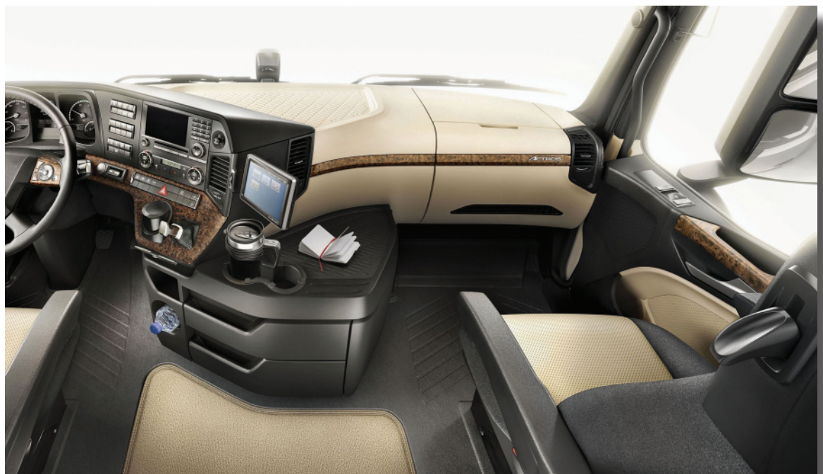
Figure 1: More comfort in the driver's cabin: blinds and covers of the new Mercedes-Benz Actros are produced with softtouch-surfaces utilizing the Dolphin-method.
