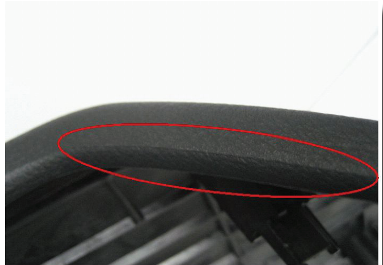
Figure 7: Modified mold design: For invisible parting lines, unobtrusive slide edges are placed.
