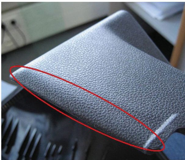
Figure 7: Modified mold design: For invisible parting lines, unobtrusive slide edges are placed.
