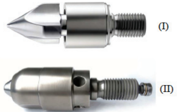
Figure 2: I) Conventional non-return valve design with 3-wing screw tip and blocking ring to prevent backflow during filling stage. II) Auto-shut-off valve (ASOV) with spring-actuated shut-off mechanism. It operates independent of screw travel with instantaneous closing and is independent of resin viscosity
