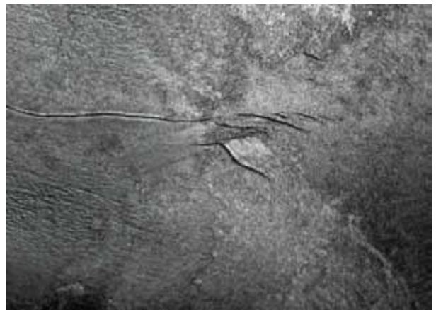
Figure 8: Higher magnification view of the cold flow markings on the right of Figure 6.
