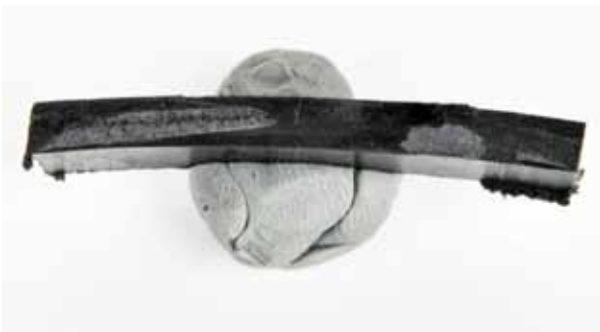
Figure 9: Photomicrograph of the defect surface from the failed support.
