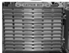
4' x 6' Ceramic Infrared Oven As shown: Operating 5 zones
