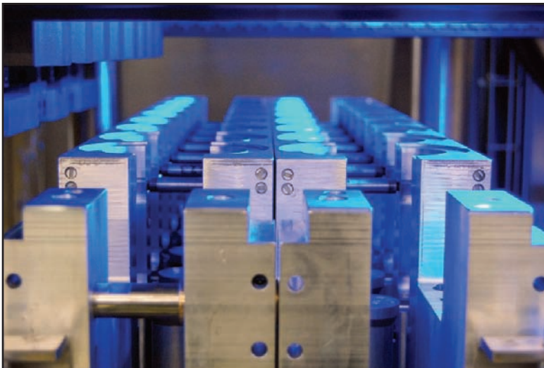
Figure 3. Detail of new tooling technology used in Illig BP70.
