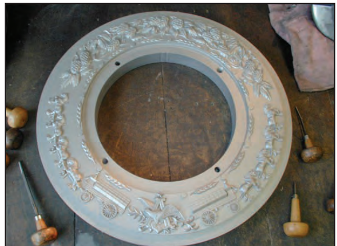
Highly detailed tooling ready to be inserted into mold
