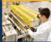
Universal anti-stat coater for top, bottom and both side coating applications
