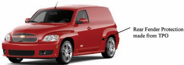
Figure 4. Chevrolet HHR with rear fender made from TPO.
