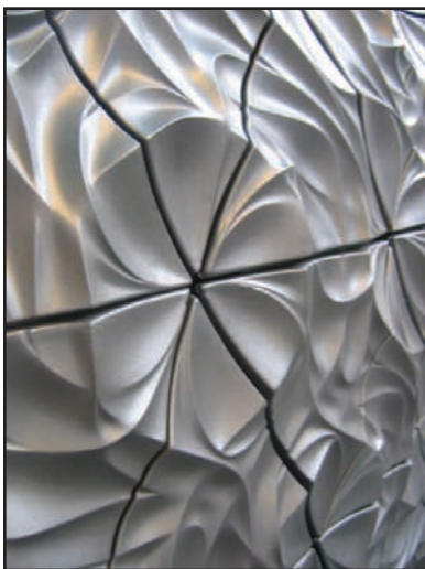
Decorative surface in PETG formed by UCLA School of Architecture and Urban Design
