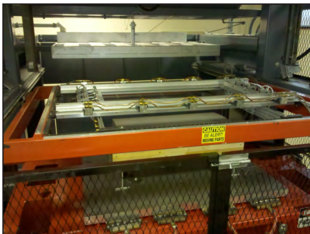
Figure 2. Renshape mold on bottom platen.
