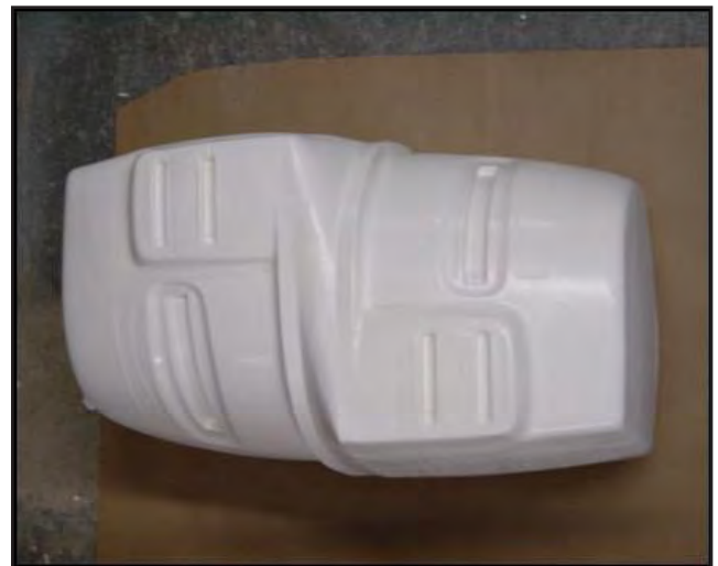
Figure 8. Finished two-part plug.
