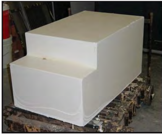
Figure 9. Near-net two-part billet.
