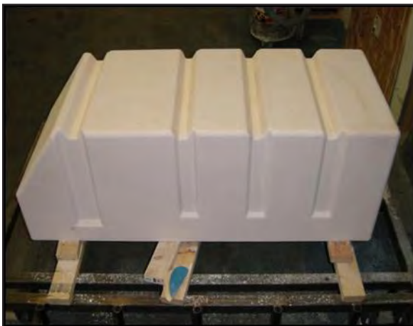
Figure 11. Syntactic foam plug for freezer liner.
