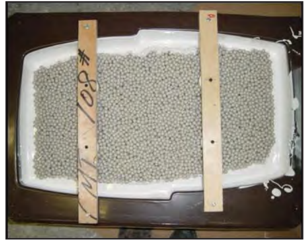
Figure 7. Syntactic is cast around and through core.
