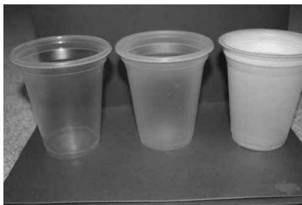
Figure 8. Non-nucleated, beta nucleated (157°C), and beta nucleated (147°C) thermoformed cups.
