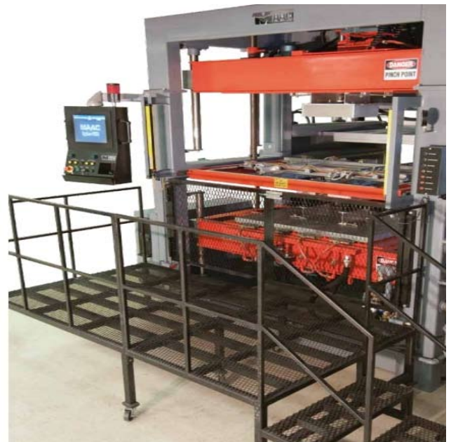
Figure 1 (1) : 890 x 1220mm MAAC thermoformer used for all testing.
