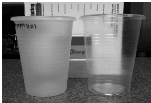
Figure 5. Beta nucleated and non-nucleated cups.
