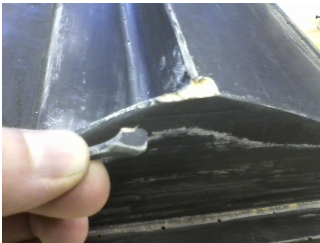
Figure 10: Broken MDF mold.
