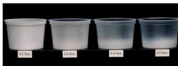
Figure 9. 16 oz. cups thermoformed at different cycle rates.
