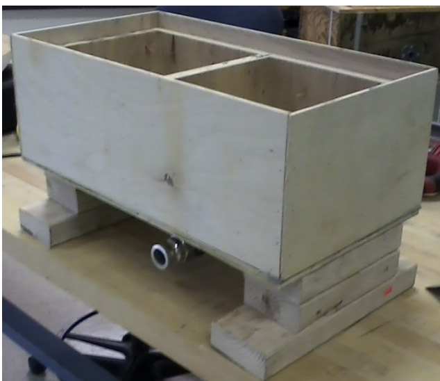
Figure 4: Vacuum box ready for mold mounting.
