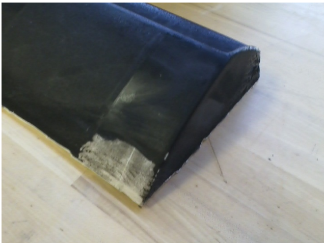
Figure 11: Failed de-molded HYTAC-C casting.
