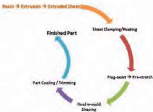
Figure 1: Schematic presentation of the plug-assist thermoforming process.
