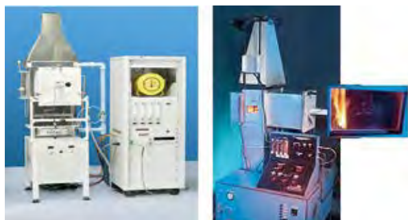
FIGURE 20 - Equipment used in FAR 25.853 testing procedure
