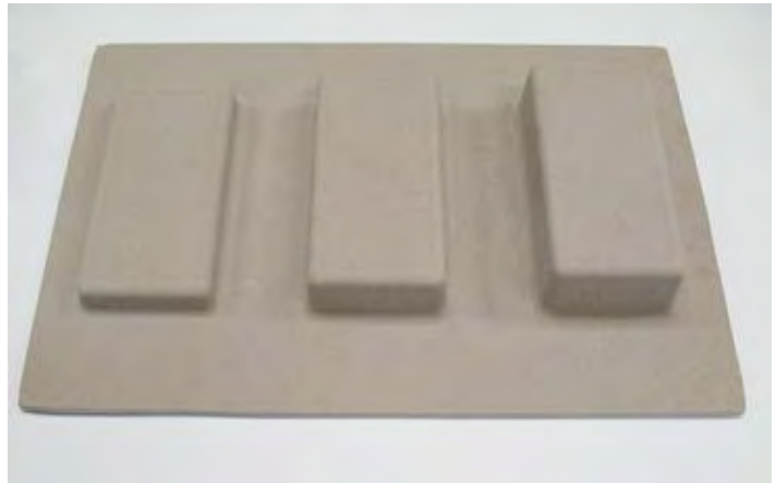
FIGURE 3. Thermoforming mold as machined for lamination trials
