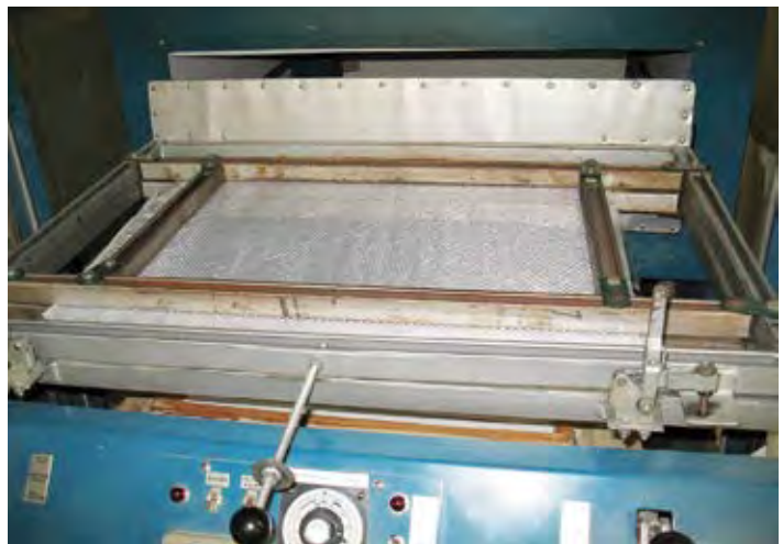
FIGURE 4. Clamped laminates prior to heating
