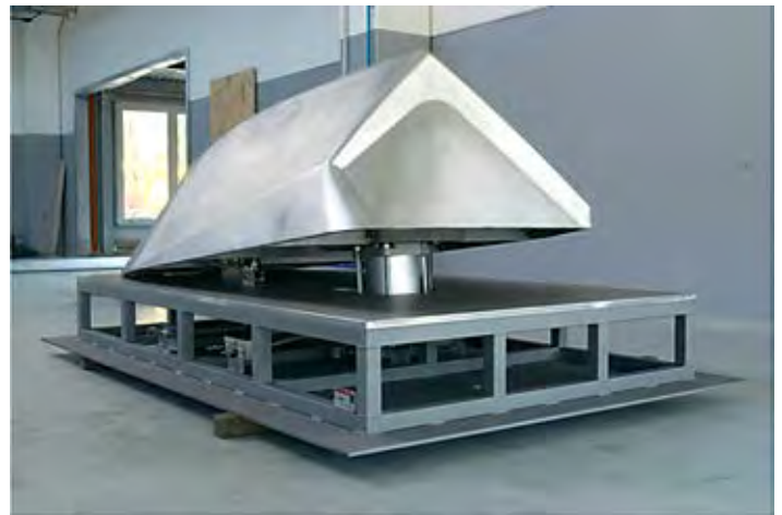
PICTURE 2: Mold Tilt to Accommodate Undercut
