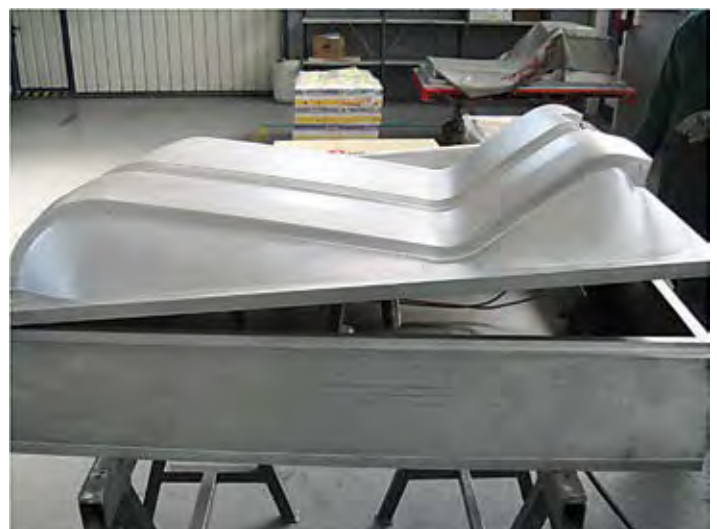
PICTURE 3: Mold Tilt to Accommodate Backdraft
