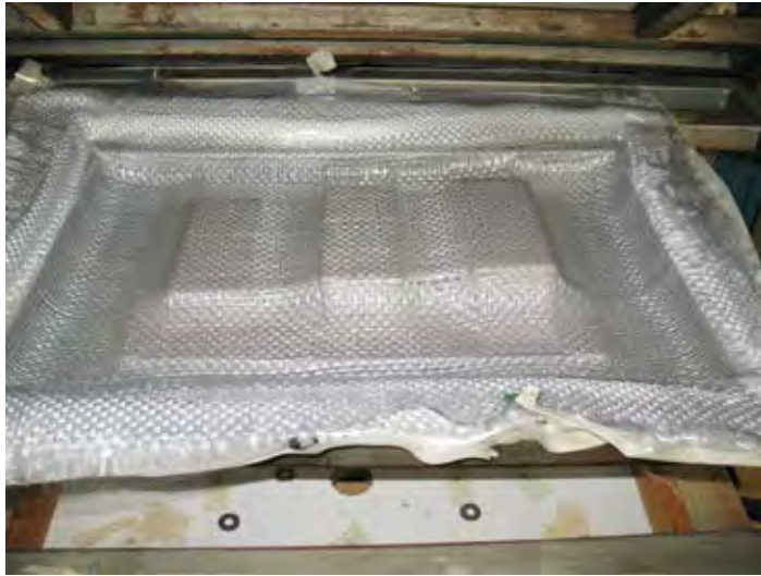
FIGURE 6. PVC-TPP60N22P lamination post-forming, prior to trim.
