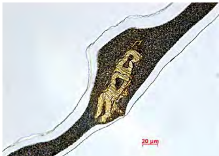
FIGURE 8. Transmitted bright-field image of PE film containing a fibrous gel.
