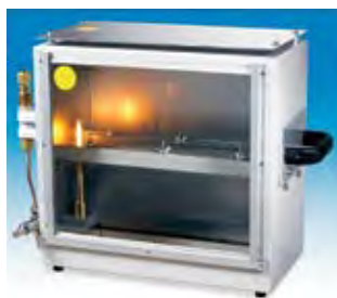
FIGURE 21 – Equipment used in FMVSS 302 flammability testing
