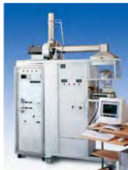
FIGURE 19 - Equipment used in ASTM E-1354 testing procedure
