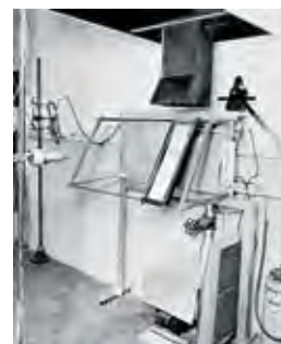
FIGURE 17 - Image of equipment used in ASTM E-162 testing procedure
