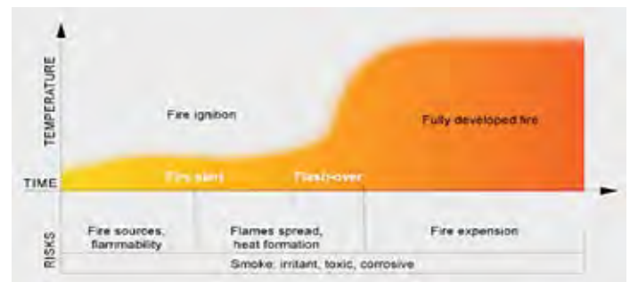
FIGURE 7 - Diagram of time vs temperature for fires
