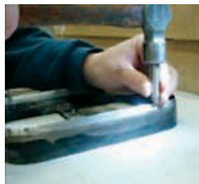
ILLUSTRATION 6: Nicking of knives to keep parts in plastic web
