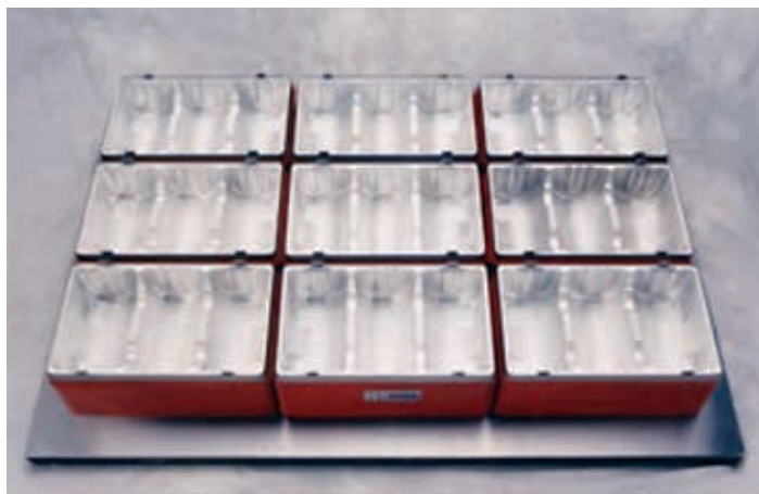
Mold cavities wrapped with forged knives courtesy of ODC Tool & Die & GN Plastics Machinery
