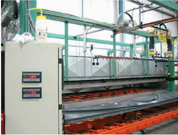
FIGURE 3. Typical plastics thermoforming machine (photo courtesy of General Plastics Machines, Ridgefield, WA).
