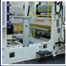
Catwalk for ease of operator access
