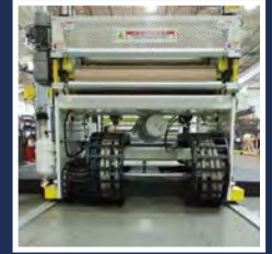
Rear positioned energy tracks permits open-side access
