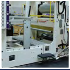
Catwalk for ease of operator access
