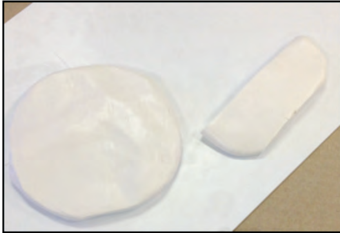
FIGURE 13: Syntactic Foam Lay-up Strips
