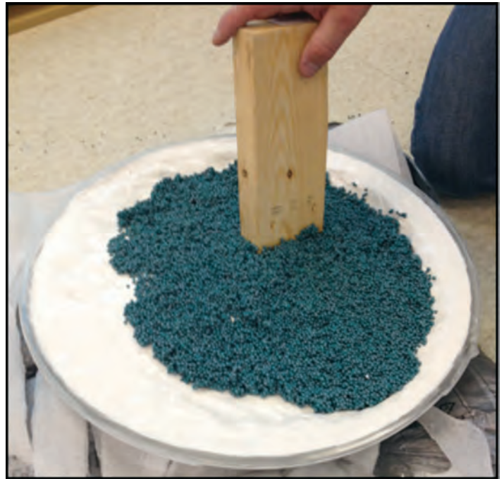
FIGURE 14: Mixed Composite beads Coated in Epoxy
