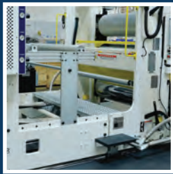
Catwalk for ease of operator access
