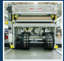
Rear positioned energy tracks permits open-side access
