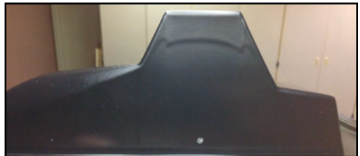
FIGURE 11: Chill Mark on KYDEX T Sheet on Aluminum mold
