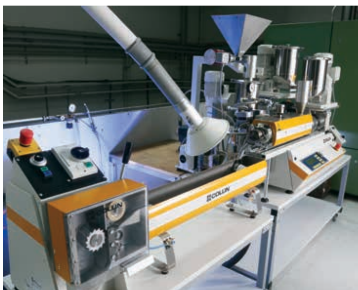
Figure 1: Co-rotating twin screw extruder at Fraunhofer IVV
