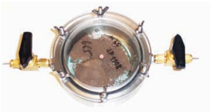
Figure 3: Measuring cell for the analysis of oxygen scavengers
