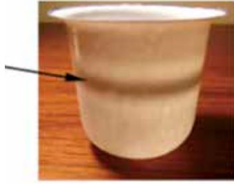
Figure 17: Uniform thickness sample with stiffening ring.
