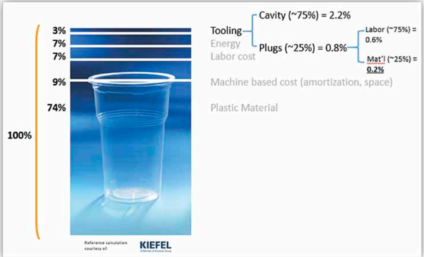
Figure 5: Illustration showing contribution to final part costs (source: Kiefel); average proportions based on industry interviews (CMT Materials data).
