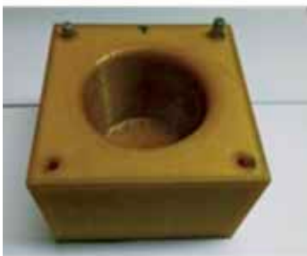
Figure 14: 3D printed mold made of Ultem.
