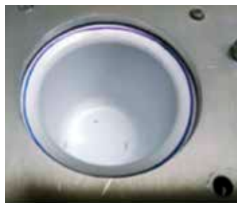
Figure 15: Vacuum thermoforming without a plug assist.
