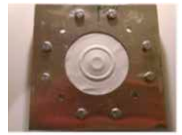
Figure 13: Quarter symmetry target model with uniform thickness = 0.010 inch.
