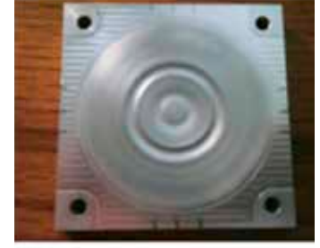
Figure 9: Bottom half of compression mold for preform design with uniform target thickness and 0.020 inch thick stiffening ring.
