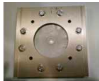
Figure 12: Quarter symmetry target model with uniform thickness = 0.010 inch.
