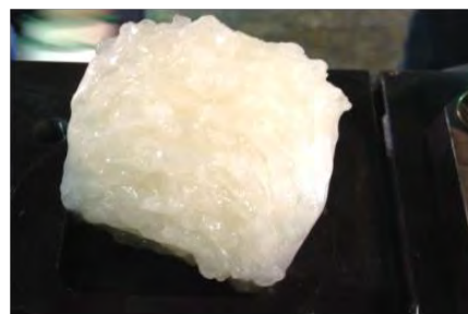
Figure 5- Melt extrudate collected from highly lubricated PLA at zone 3 Figure 1- Image of melt extrudate removed from zone 3 on screw design #1.
