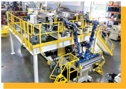
Special low-friction adapter piping and sheet die feature insulation blankets for high energy efficiency and operator safety.
