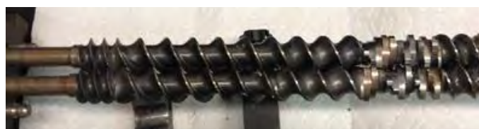
Figure 6- Melting region of screw design 1 using GFF screw elements and kneading blocks in zone 2.
