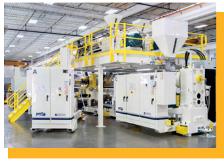
Low-boy co-extruders positioned on a mezzanine assure easy operator access to the extrusion complex and a compact footprint.
