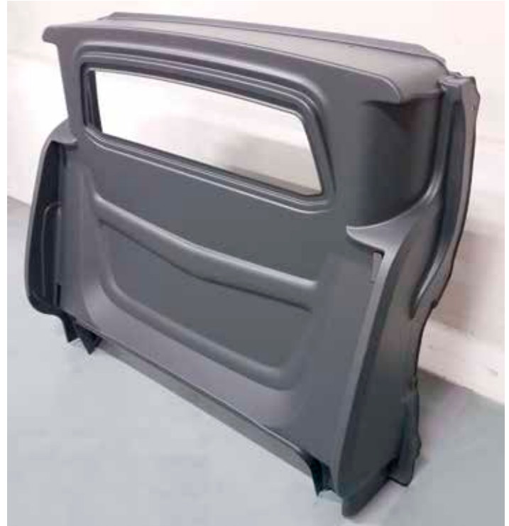
Image 4: Heavy Gauge Part Competition Winner (Automotive): RPC Promens (Kópavogur, Iceland) This interior door demonstrates very complex shapes - high pre-blow (600 mm) prior to forming. This part is deemed a high security part according to ISO 27956. (Courtesy RPC Promens)
