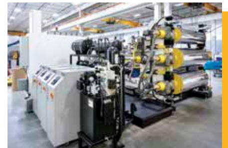
G-SERIES® configurable 5-roll compact vertical roll stand features high efficiency temperature control modules and open operator access.
