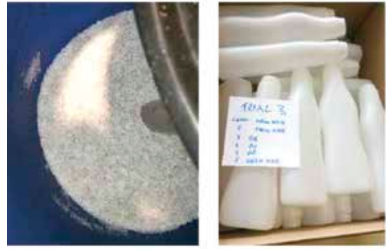
Figure 4: Blend A dry mixed 1:1 with vHDPE (LHS) Bottles produced from trial #3 (RHS)
