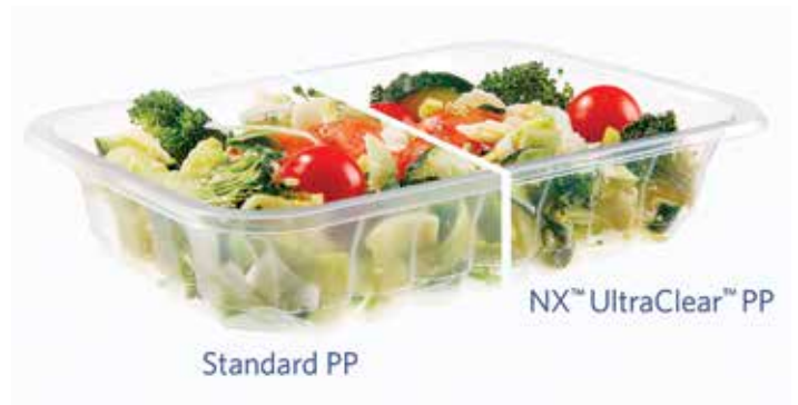
Image 5: Thin Gauge Part Competition Winner: Milliken Chemical (Spartanburg, SC, USA) PP tray from Milliken illustrated weight reduction from 14g to 12g tray (16%) while maintaining optical clarity and improving impact strength over PET version. (Courtesy Milliken Chemical)
