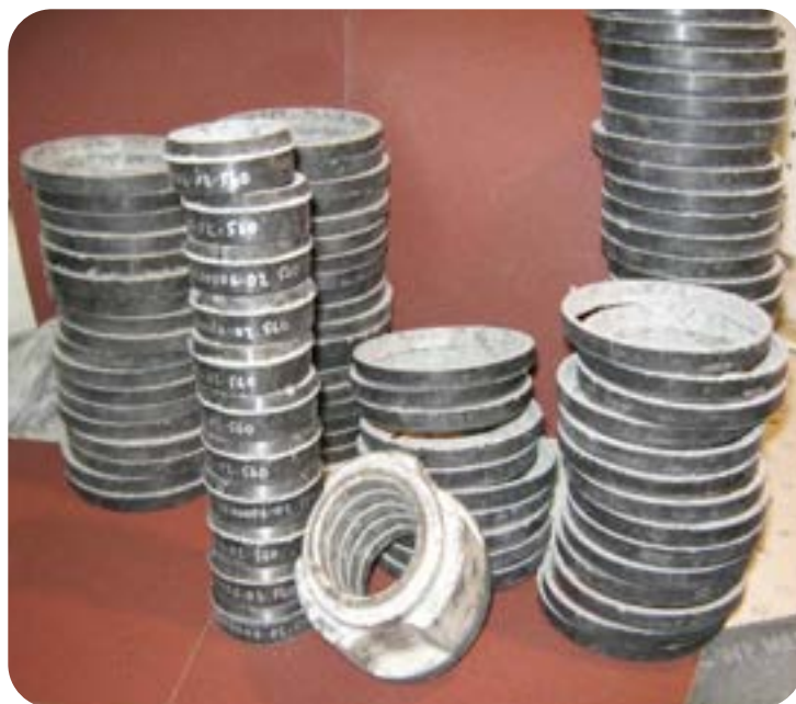
molded and machined Kevlar-based wear rings
