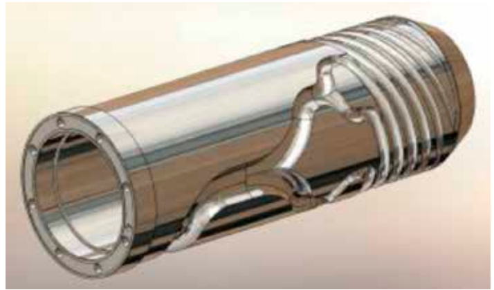
Figure 5: Significantly more performance in extrusion blow molding due to BEKUM high-tech spiral distributor extrusion heads.
