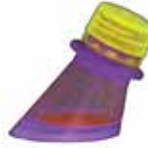
Figure 2: The Zeiss software uses color to show different parts (densities) of the assembly. Color transparency is added to accentuate details further.
