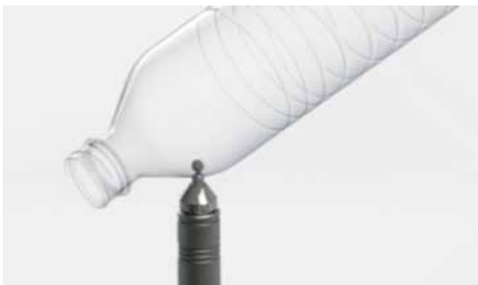
Figure 1: A Magna Mike probe can be used to measure only the overall wall thickness .
