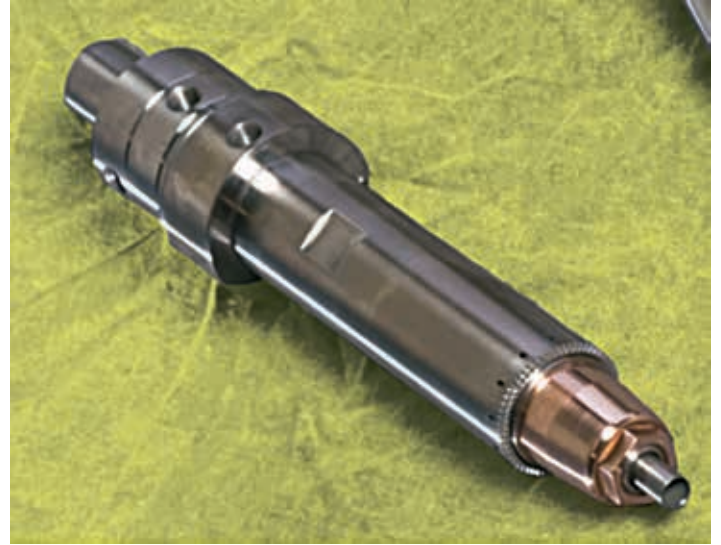
Figure 4: Direct Water Cooled; with Recirculating air
