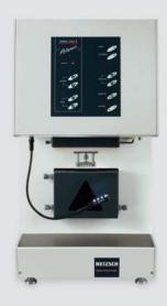
**Dynamic Mechanical Analysis** (DMA) to characterize stiffness and damping behavior
