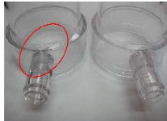
Figure 5. Dialyzer housings after exposure to Virex TB™. The PC housing on the left shows a significant crack (visible in the circled area) after 8 hours exposure. The Tritan™ housing on the right has not cracked after 120 hours exposure.
