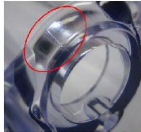
Figure 4. PC medical device after exposure to 24 hours of isopropyl alcohol. A large crack is visible in the circled area.
