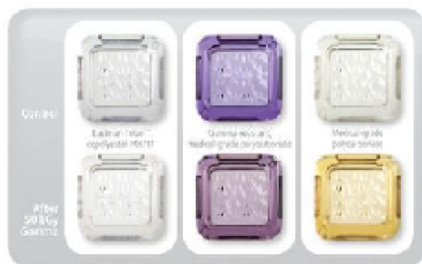
Figure 1. Color shift measured using CIELAB color ( b^* ) and photography after 50 kGy of e-beam radiation for samples of Tritan™ MX711, gamma resistant PC and standard grade PC and acrylic. Positive and negative b^* values correspond to a yellow and blue hue, respectively.
