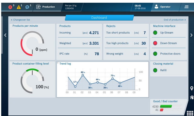
Condition monitoring delivers info on the individual machines or complete lines in real time. Based on pre-defined alarm and failure limits deviations can be detected and eliminated early on.
